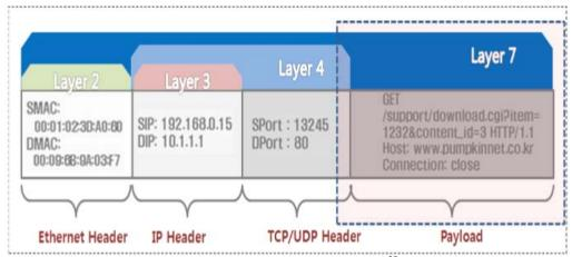
Figure I: Packet Inspection models<sup>20</sup>
